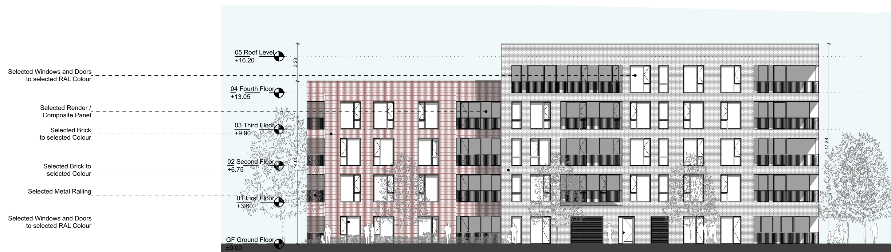
1:200 East Elevation - Facing Open Space
